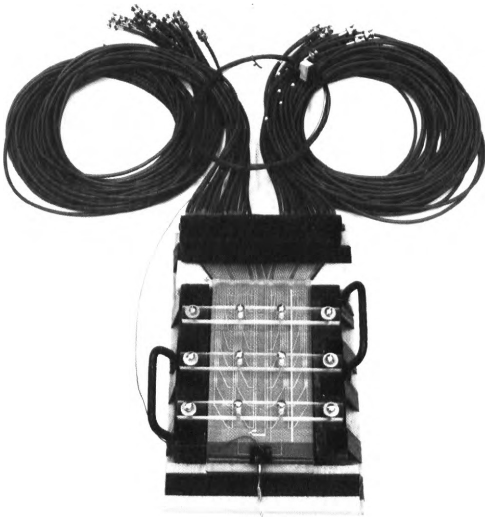
Fig. 2. Detonation velocity block test fire assembly.
